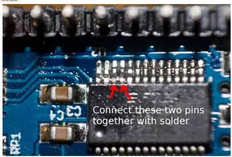
Notice which two pins have solder between them. You should check connection with multimeter. This fix needs some good eye-hand coordination as parts are kinda tiny. Pin pitch in this
