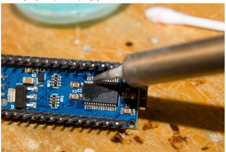
Touch touch 3th and 4rd IC pins from the left with a hot wet soldering iron tip. You need to bridge these pins together. Be careful not to solder any other pins or damage the Arduino
